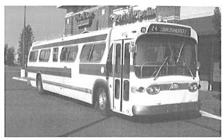
The 40' semi-suburbans had 8V-71 engines and VS-2 transmissions, and all were 96" wide. Each had single doors with all forward facing reclining seats built to seat 45 but later converted to 49 passengers. These units were in the 800 series and Tom owns ex #810.
